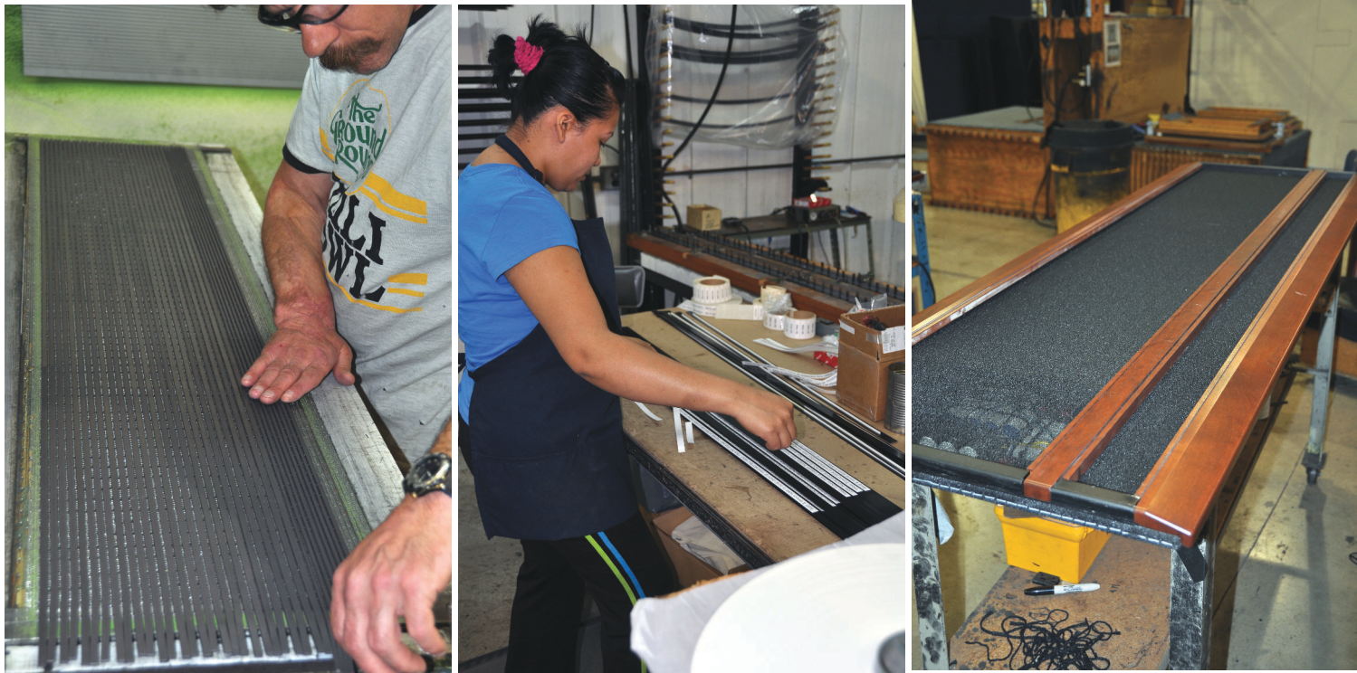
Magnet structure of a Magnepan panel.
